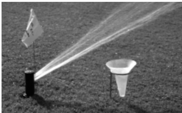
Place the catch can far enough away from the sprinkler head to avoid obstructing the spray pattern.
