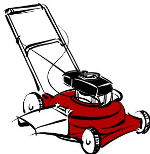
a clutch handle or switch that stops the blade within 3 seconds after the operator lets go.
