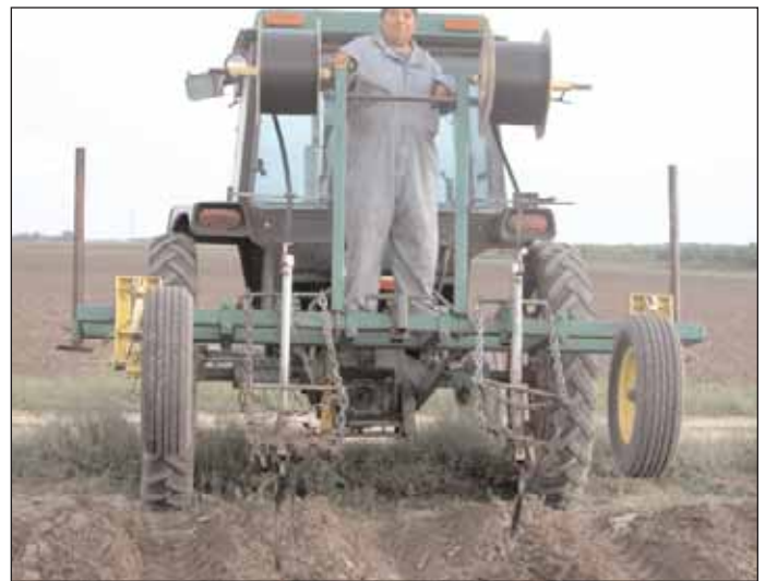
Figure 3. Toolbars with drip tape injector.
