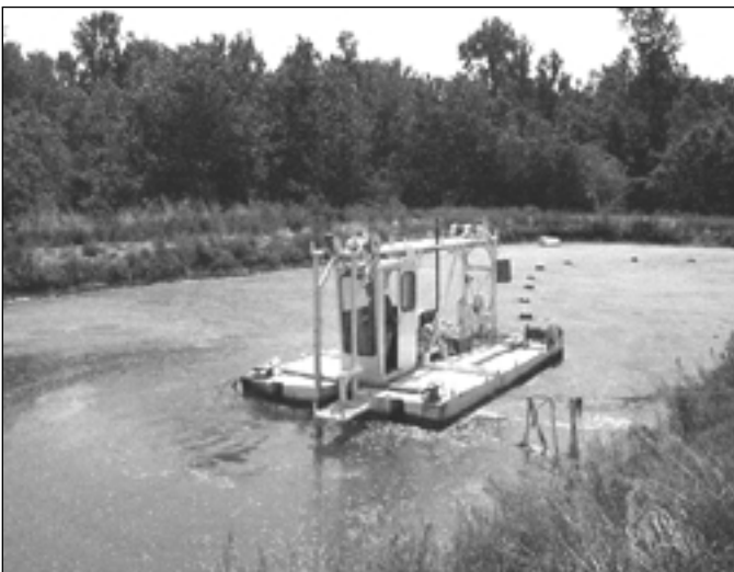
Figure 2. Pumping dredge operating in a lagoon.
