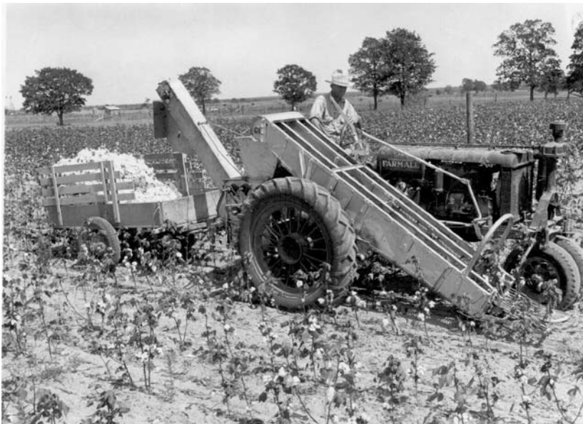
Fig. 5.4, The Texas State Cotton Harvester schematic showing the stripping rolls, conveying and burr extraction mechanism for the 1938 design.
